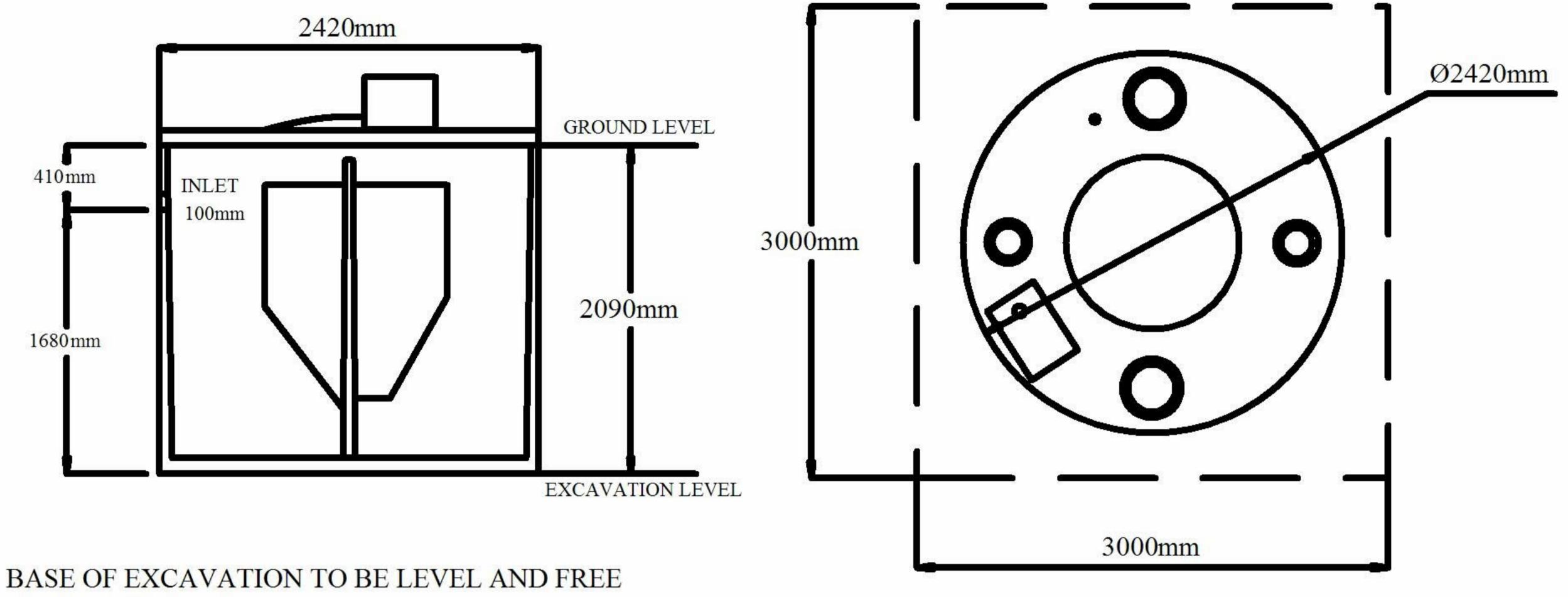
BASE OF EXCAVATION TO BE LEVEL AND FREE OF BROKEN ROCK
