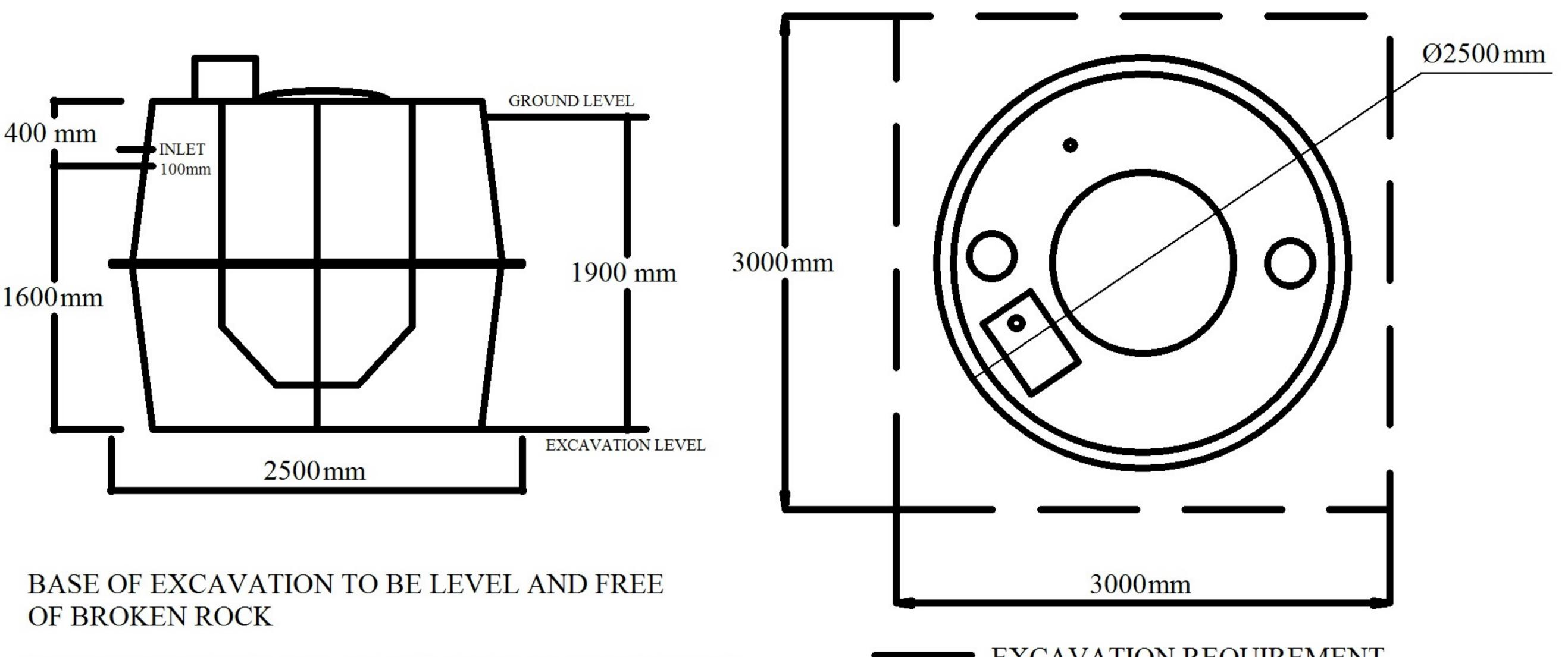
IF REQUIRED PREPARE A BASE OF 12mm SCREENINGS, DOLOMITE OR CONCRETE
