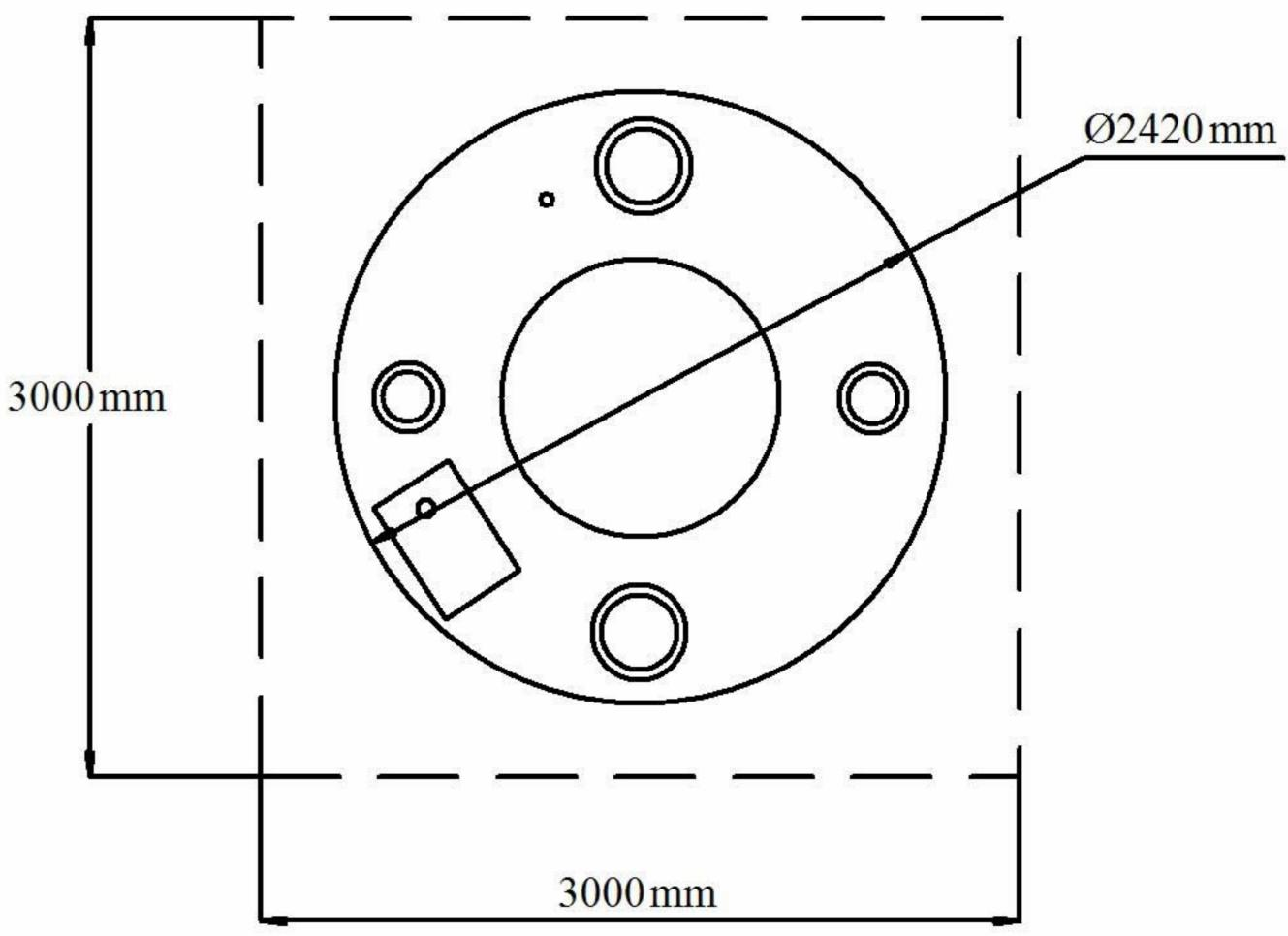
BASE OF EXCAVATION TO BE LEVEL AND FREE OF BROKEN ROCK
